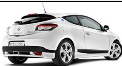
Hatchback/ Liftback 3 or 5 door car, in which back seats fold down to create more cargo space
